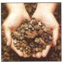
The strength of ESCS aggregates aids the SmartWall CMU's chipping resistance.
